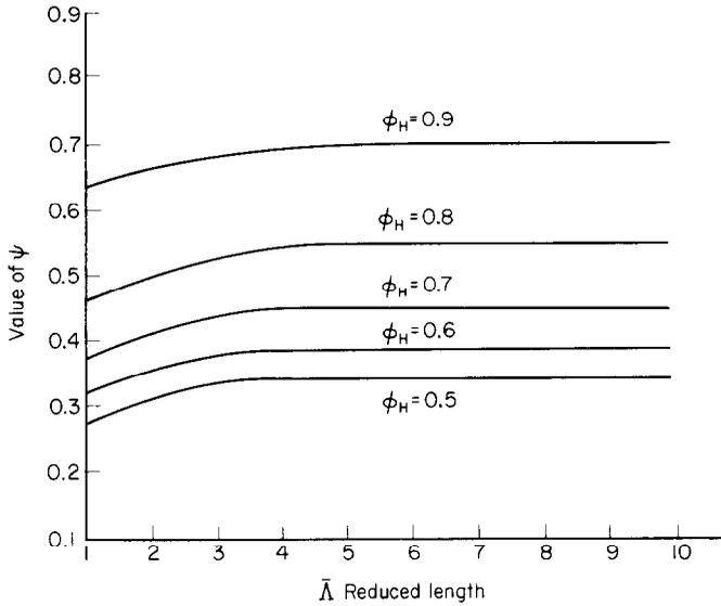
FIG. 3. Variation of  $\psi$  with respect to reduced length  $\bar{\Lambda}$  and the Hausen  $\phi_H$  factor.
