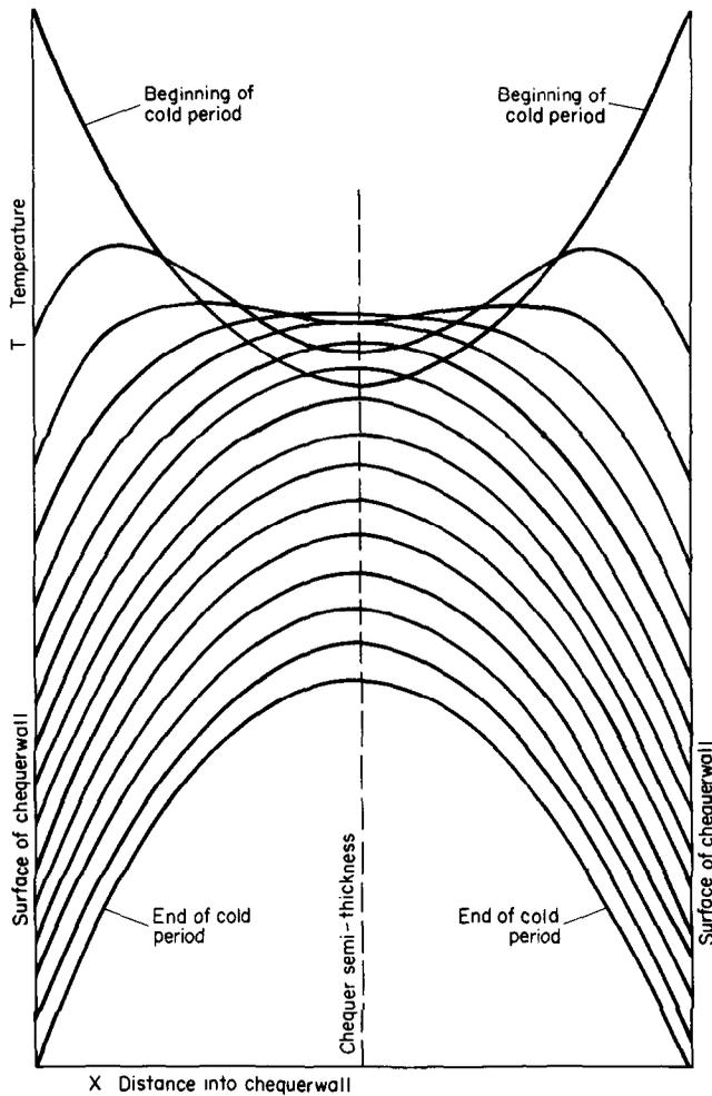
FIG. 1. Solid temperature profile changes as a period of operation progresses.
