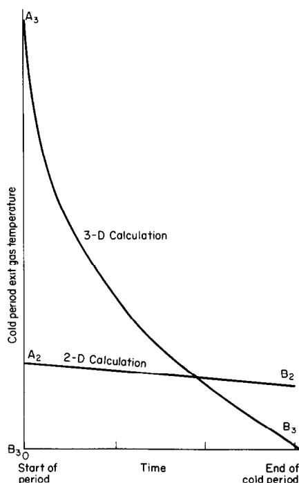
FIG. 2. Comparison between exit gas temperatures computed using 3-D equations and using 2-D equations.
